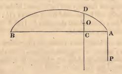
Let w = weight of the string. L = length. D d : L : : weight D d : w  $\therefore$  weight of D d =  $\frac{D d \times w}{L}$  Also
